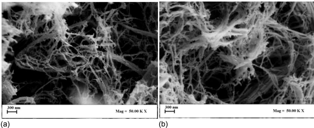
*Figure 4: SF+AA aerogels processed at 200 bar, 35 °C for 4 h: (a) 10 % w/w SF; (b) 15 % w/w SF.*
