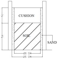
Figure 1. Schematic representation of sample preparation of soilcushion layers for test
