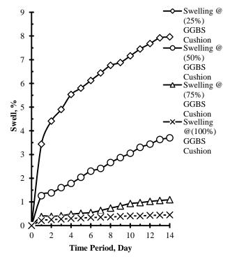
Figure 2. Swell behaviour of expansive soil with different thickness of lime treated GGBS cushion
