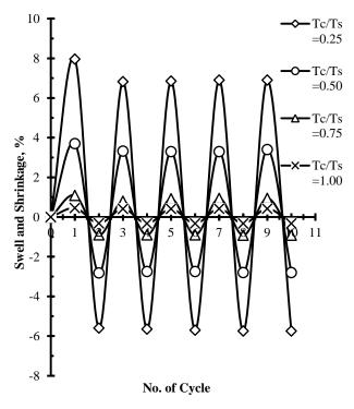
Figure 3. Cyclic swell-shrinkage behaviour of expansive soil with different thickness of lime treated GGBS cushion
