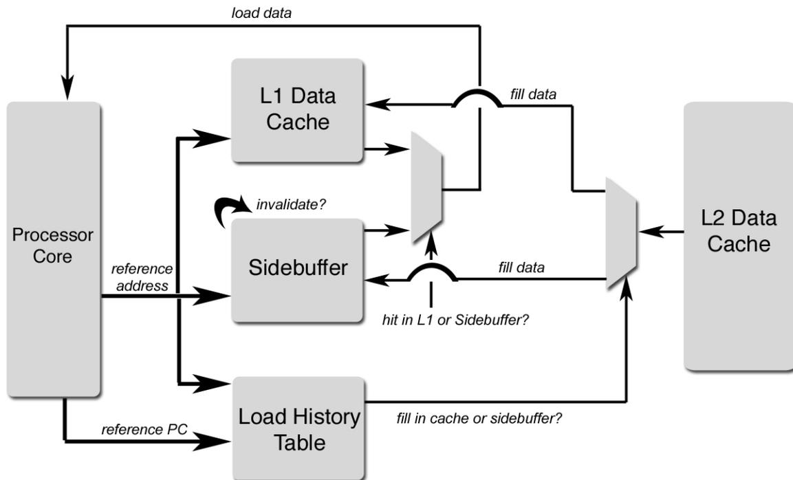
Figure 4: Dynamic Cache Allocation Architecture
