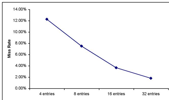
Figure 7: Effect of Sidebuffer Size on Combined L1/Sidebuffer Miss Rate (gzip-graphic)
