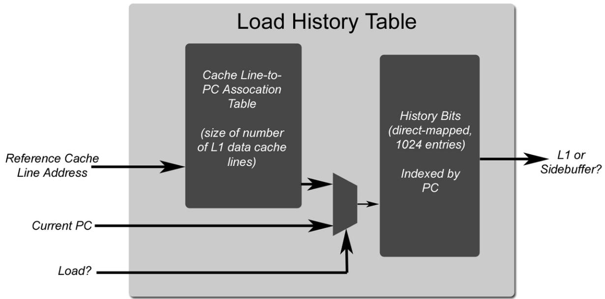
Figure 5: Internal LHT Architecture
