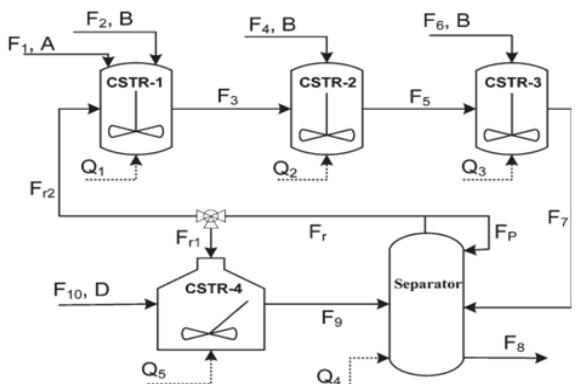
Figure 3. Flow Diagram of Alkylation of Benzene Process Plant
