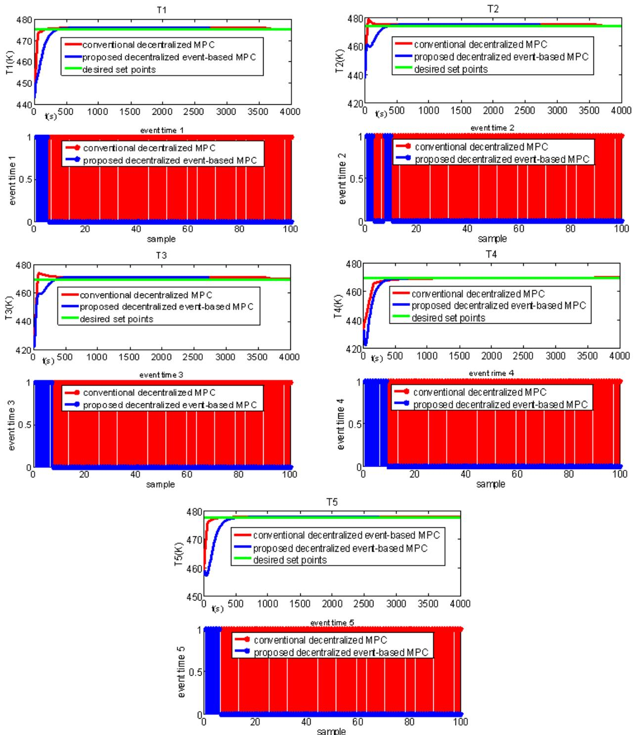
**Figure 4.** comparative plant outputs due to both the decentralized event-based MPC and the decentralized MPC exercised on the Alkylation of Benzene process plant
