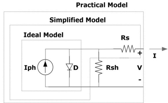
Figure 2. Equivalent circuit of PV cell [13]
