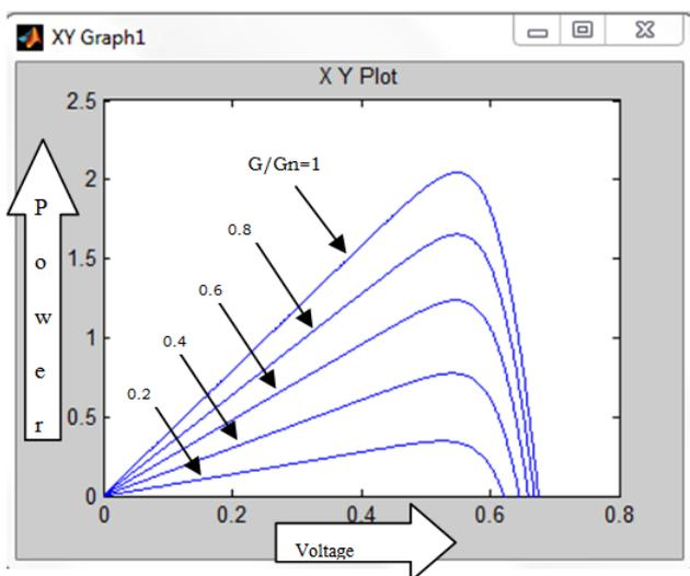
Figure 4. P-V characteristics of the cell for variation of the solar irradiance
