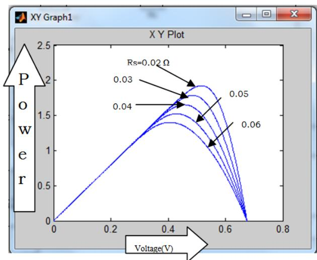
Figure 5. P-V characteristics of the cell for variation of the series resistance
