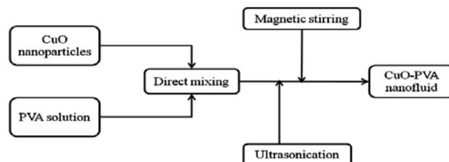
Figure 1. Preparation of CuO-PVA nanofluid
