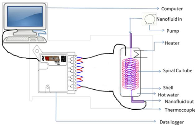
Figure 4. Experimental setup for the measurement of forced convective heat transfer coefficient of nanofluids
