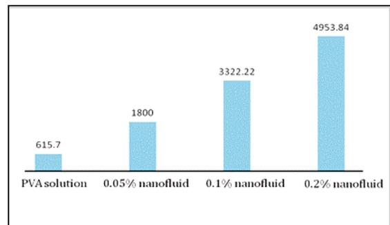
Figure 5. Forced convective heat transfer coefficient in W/(m<sup>2</sup>K) of PVA solution and CuO-PVA nanofluids
