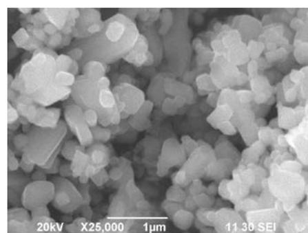
Figure 3. SEM image of CuO-NPs
