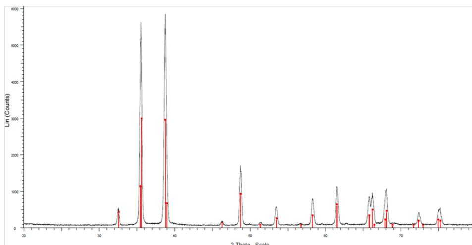
Figure 2. XRD pattern of CuO NPs. The (|) vertical lines indicate the position and relative intensity of 05-0661 JCPDS card file diffraction peaks for the monoclinic phase
