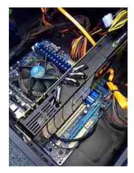
Figure 19.1: GTX 480 GPU (top of the line in 2010!)
