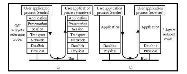
**Fig. 1.8.** The OSI 7-layers reference model (a), and the reduced fieldbus 3-layer structure (b).
