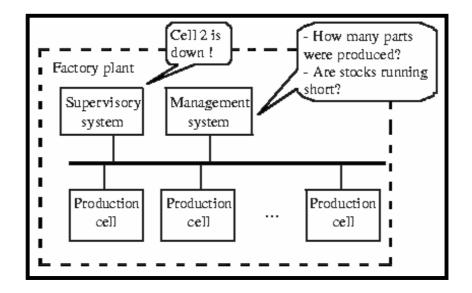
**Fig. 1.5.** The trend towards the use of a distributed architecture in manufacturing industry to interconnect cells across the plant.
