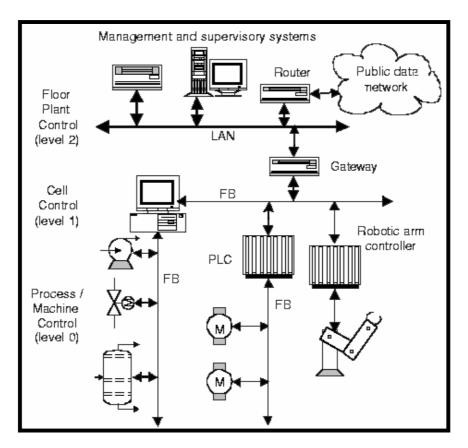
Fig. 1.6. The Computer Integrated Manufacturing (CIM) Architecture.
