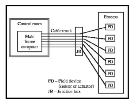
**Fig. 1.1.** Star topology typically used in the architecture of Process Control Systems up to the 1960s.
