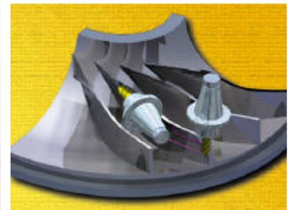
(F) Multi axis and multi spindle milling
