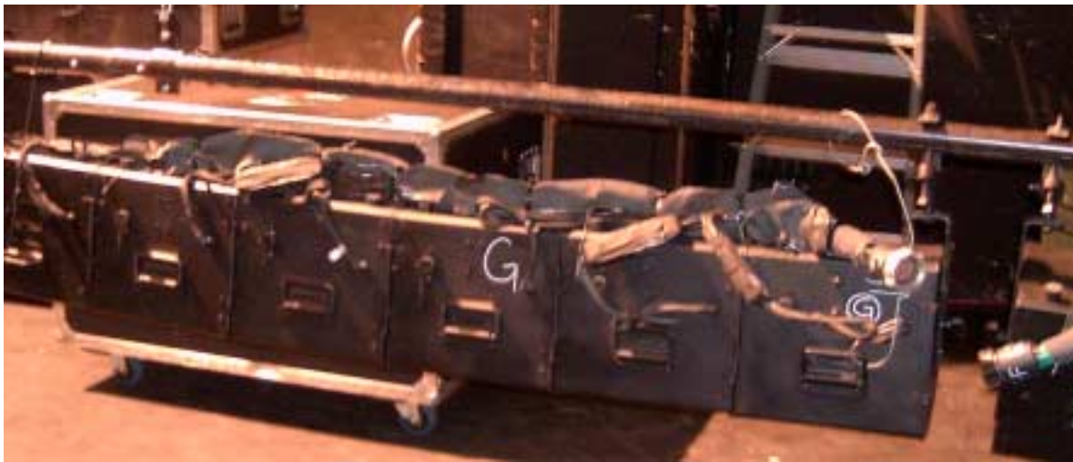
Economy Striplights barrel bolted together to form a five-unit strip. Note the letter "G" that indicates it is the seventh unit from SL and the "fist" space between the units
