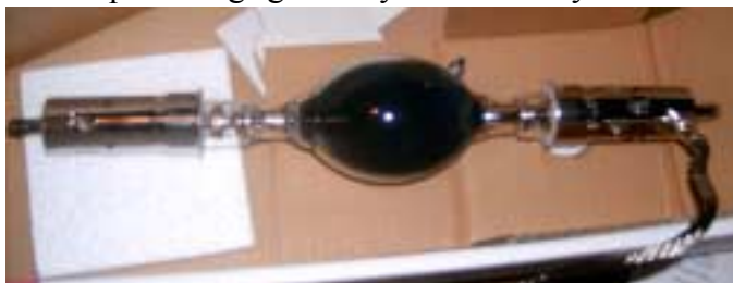
3K Xenon Lamp from a Lycian 1293 that burned out. Note the black envelope surrounding the anode and cathode. You can also see the Lamp seal or PST, upper right of lamp
