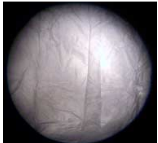
Above is a bad bench focus; note the hot spot in the upper right corner of the field.
