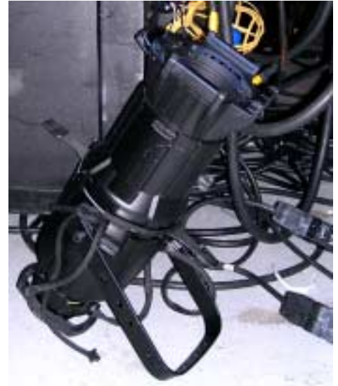
Modern "Ghost Load" used with Dimmable Fluorescents
