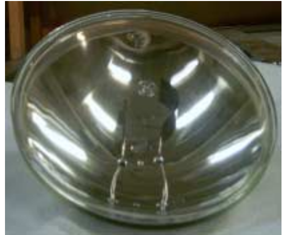
Aircraft Landing Light, abbreviated ACL, note filament and reflector
