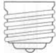
Mogul Screw E39 (38.3mm screw)
