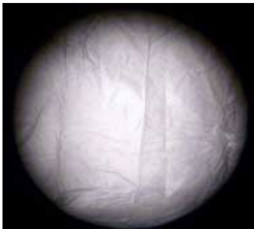
Above is a good bench focus, with a relatively flat field (even & bright).
