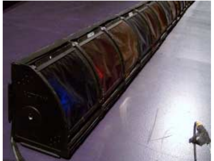
Economy Strips used as a Ground Row UPS
