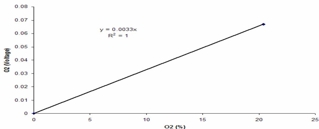
**Figure 2.3** Calibration of oxygen probe, (A) the arrow is indicates the time of the addition of NaSCN, AA, and NaNO<sub>2</sub> and (B) obtaining a linear response between electrical signals of O<sub>2</sub> (volts) and O<sub>2</sub> levels (%).
