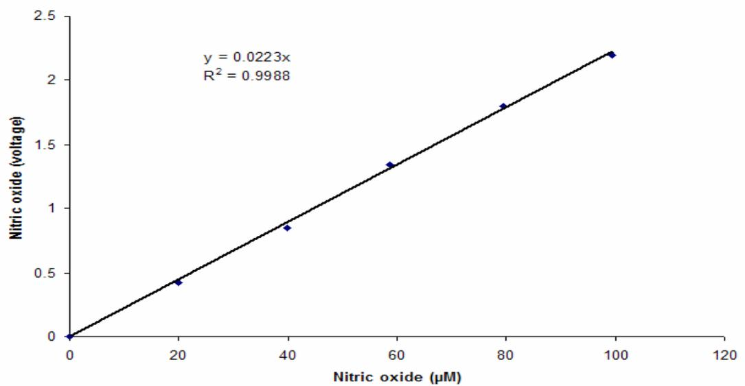
Figure 2.2 Calibration of nitric oxide probe, (A) by adding successive bolus dose of 50µl NaNO<sub>2</sub> to sulphuric acid (0.1M) containing potassium iodide (0.1M), and (B) obtaining a linear response between electrical signal of NO (volts) and NO concentration (µM).
