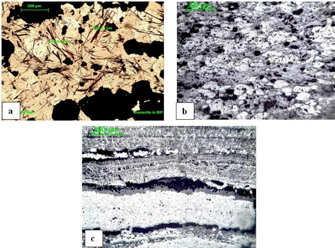
**Figure 3.** Photomicrographs showing (a) Grunerite with magnetite in BIF-I, (b) magnetite and martite in elongated form in BIF-II, (c) Hematite diagenetically grows in bands of BIF-III (Leica DM 2500 P)
