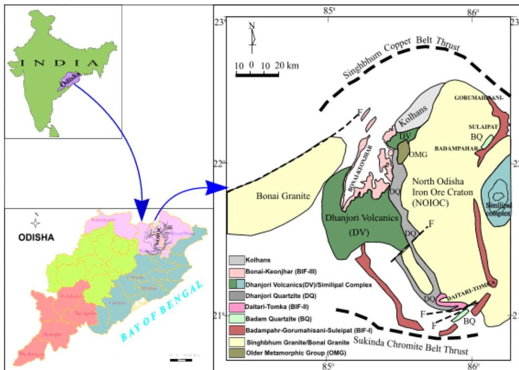
**Figure 1.** Generalised geological map showing BIF-I, BIF-II and BIF-III surrounding the North Odisha Iron Ore Craton (NOIOC) (Modified after [20,26])
