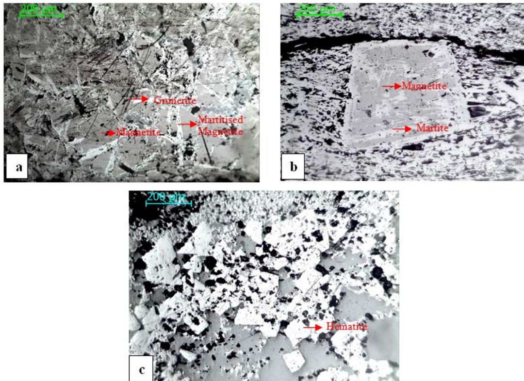
**Figure 4.** Photomicrographs showing (a) Grunerite, magnetite (primary) and martitised magnetite in BIF-I, (b) Magnetite and martite in BIF-II, (c) Hematite in BIF-III
