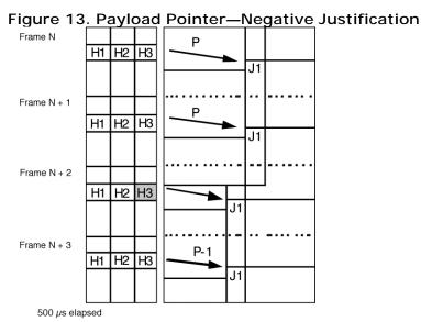
The SPE moves forward in time when a data byte has been stuffed into the H3 byte.
