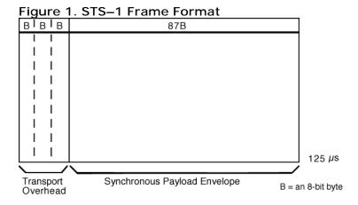
The synchronous payload envelope can also be divided into two parts: the STS path overhead (POH) and the payload. The payload is the revenue-producing traffic being transported and routed over the SONET network. Once the payload is multiplexed into the synchronous payload envelope, it can be transported and switched through SONET without having to be examined and possibly demultiplexed at intermediate nodes. Thus, SONET is said to be service-independent or transparent.
