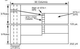
Figure 11. Pointer—SPE Position in the STS-1 Frame
