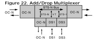
A single-stage multiplexer/demultiplexer can multiplex various inputs into an OC-N signal. At an add/drop site, only those signals that need to be accessed are dropped or inserted. The remaining traffic continues through the network element without requiring special pass-through units or other signal processing.
