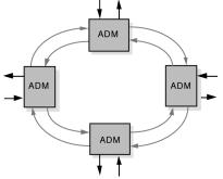
The demand for survivable services, diverse routing of fiber facilities, flexibility to rearrange services to alternate serving nodes, as well as automatic restoration within seconds, have made rings a popular SONET topology.
