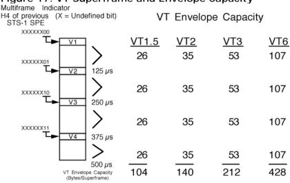
Figure 17. VT Superframe and Envelope Capacity
