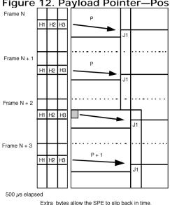
Figure 12. Payload Pointer—Positive Justification
