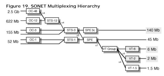
Except for concatenated signals, all inputs are eventually converted to a base format of a synchronous STS-1 signal (51.84 Mbps or higher). Lower-speed inputs such as DS-1s are first bit- or byte-multiplexed into VTs. Several synchronous STS-1s are then multiplexed together in either a single- or two-stage process to form an electrical STS-N signal (N>=1).
