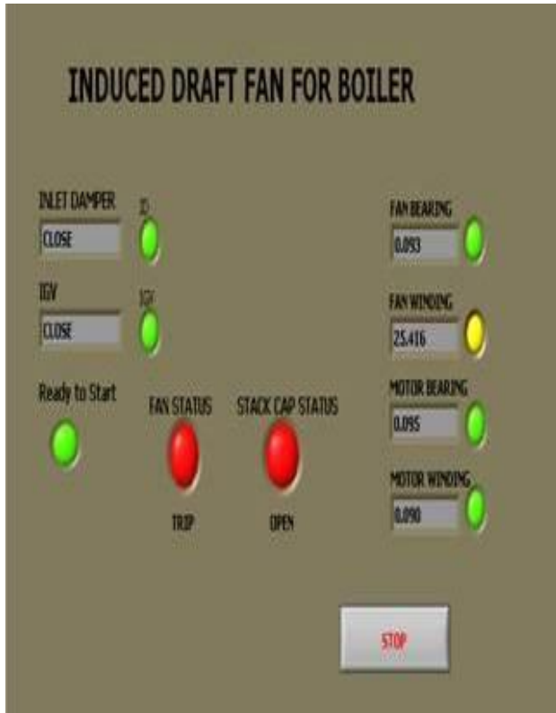
Fig-10 Fan Winding Temperature beyond limit
