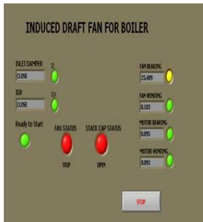
Fig-9 Fan Bearing Temperature. Beyond limit
