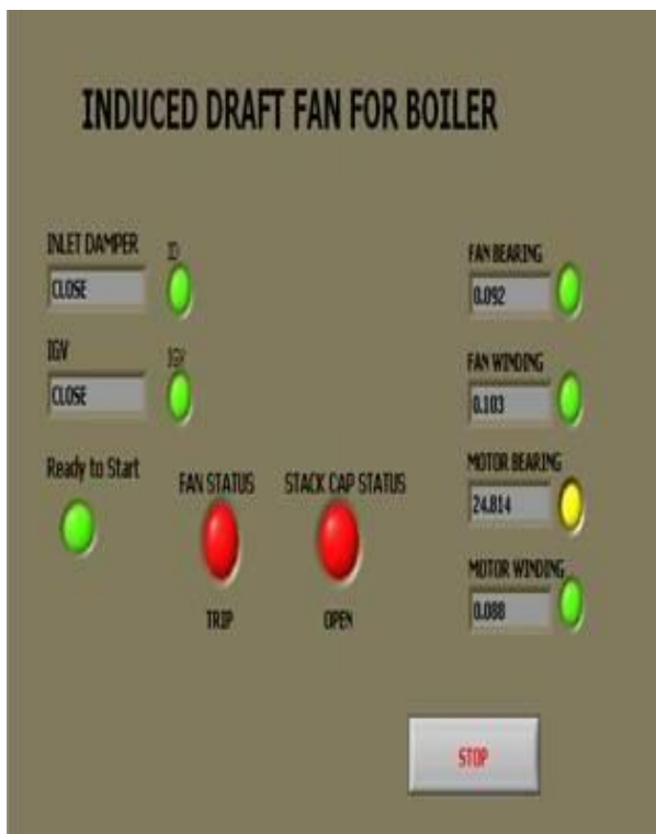
Fig-11 Motor Bearing Temperature beyond limit
