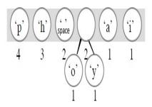
Figure 1b. First tree root of Huffman's code
