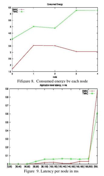
out policy of T Mac get insignificant..Figure 9 shows the application level latency for all the five nodes in wireless sensor network. S Mac protocol faces severe packet failure in non reception mode. The effect of interference is minor in both the protocols because the sensor nodes in this arrangement are kept far from each other.
