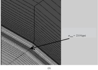
Resorting to another source,<sup>13</sup> the stress concentration factor is found to be  $K_t = 3.00$ . The reaction at the right support is  $R_F = (8/20)600 = 240$  lbf. The bending moment at the start of the fillet is M = 240(11.52) = 2765 lbf · in = 2.765 kip · in. The analytical prediction of the maximum stress is thus
