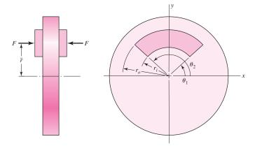
of a rotating disk. Depicted in Fig. 16-19 is the geometry of an annular-pad brake contact area. The governing axial wear equation is Eq. (12-27), p. 643,
