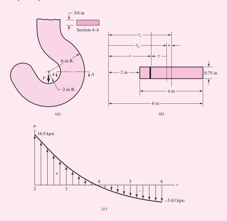
Note in the hook example, the symmetrical rectangular cross section causes the maximum tensile stress to be 3 times greater than the maximum compressive stress. If we wanted to design the hook to use material more effectively we would use more material at the inner radius and less material at the outer radius. For this reason, trapezoidal, T, or unsymmetric I, cross sections are commonly used. Sections most frequently encountered in the stress analysis of curved beams are shown in Table 3–4.
