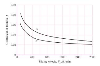
Published values of the coefficient of friction vary as much as 20 percent, undoubtedly because of the differences in surface finish, materials, and lubrication. The values on the chart of Fig. 13–42 are representative and indicate the general trend.
