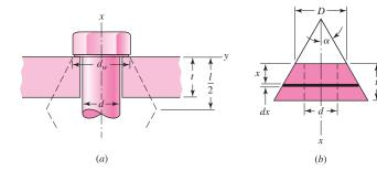
The pressure, however, falls off farther away from the bolt. Thus Ito suggests the use of Rotscher's pressure-cone method for stiffness calculations with a variable cone angle. This method is quite complicated, and so here we choose to use a simpler approach using a fixed cone angle.
