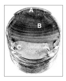
a sudden, fast fracture. A stage III fracture can be brittle, ductile, or a combination of both. Quite often the beach marks, if they exist, and possible patterns in the stage III fracture called *chevron lines*, point toward the origins of the initial cracks.
