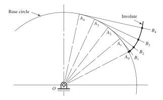
First, it is necessary to learn how to construct an involute curve. As shown in Fig. 13–8, divide the base circle into a number of equal parts, and construct radial lines  $OA_0$ ,  $OA_1$ ,  $OA_2$ , etc. Beginning at  $A_1$ , construct perpendiculars  $A_1B_1$ ,  $A_2B_2$ ,  $A_3B_3$ , etc. Then along  $A_1B_1$  lay off the distance  $A_1A_0$ , along  $A_2B_2$  lay off twice the distance  $A_1A_0$ , etc., producing points through which the involute curve can be constructed.
