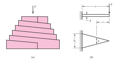
which is proportional to the distance x if I/c is a constant. But there is no reason why I/c need be a constant. For example, one might design such a spring as that shown in Fig. 10–14b, in which the thickness h is constant but the width b is permitted to vary. Since, for a rectangular section,  $I/c = bh^2/6$ , we have, from Eq. (a),
