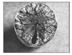
Failures Resulting from Static Loading
