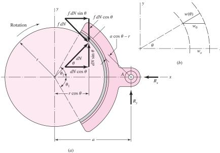
where K is a material constant, P is pressure, V is rim velocity, and t is time. Then, denoting P as  $p(\theta)$  above and solving for  $p(\theta)$  gives
