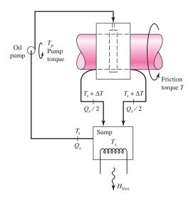
Equating the heat gain to the frictional work and solving for  $\Delta T$  gives
