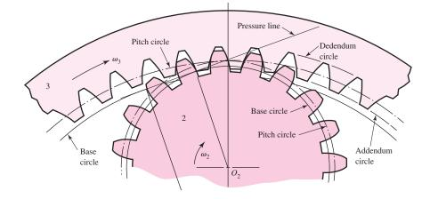
Thus the pitch circles of gears really do not come into existence until a pair of gears are brought into mesh.
