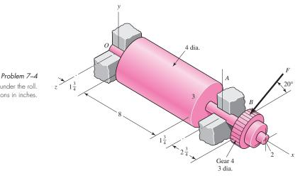
**7–5** Design a shaft for the situation of the industrial roll of Prob. 7–4 with a design factor of 2 and a reliability goal of 0.999 against fatigue failure. Plan for a ball bearing on the left and a cylindrical roller on the right. For deformation use a factor of safety of 2.
