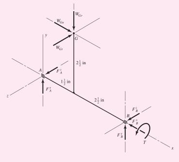
These three components are now inserted on the sketch as shown at B in Fig. 13–44. Summing forces in the y direction,
