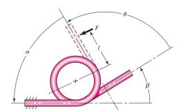
where  $N_p$  is the number of partial turns. The above equation means that  $N_b$  takes on noninteger, discrete values such as 5.3, 6.3, 7.3, ..., with successive differences of 1 as possibilities in designing a specific spring. This consideration will be discussed later.
