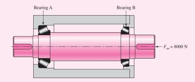
Noting that  $F_{ae}$  to the right is positive (Table 11–6), with direct mounting m = +1, we can write
