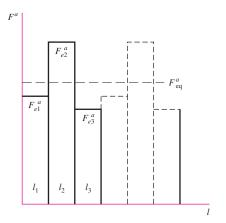
Consider the piecewise continuous cycle depicted in Fig. 11–10. The loads  $F_{ei}$  are equivalent steady radial loads for combined radial–thrust loads. The damage done by loads  $F_{e1}$ ,  $F_{e2}$ , and  $F_{e3}$  is
