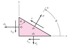
Equation (3–10) defines two particular values for the angle  $2\phi_p$ , one of which defines the maximum normal stress  $\sigma_1$  and the other, the minimum normal stress  $\sigma_2$ . These two stresses are called the *principal stresses*, and their corresponding directions, the *princi*pal directions. The angle between the principal directions is 90°. It is important to note that Eq. (3–10) can be written in the form
