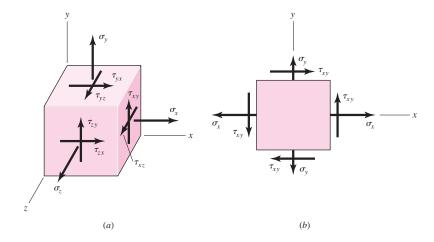
dimensions of the cube in Fig. 3–8*a* approach zero, the stresses on the hidden faces become equal and opposite to those on the opposing visible faces. Thus, in general, a complete state of stress is defined by nine stress components,  $\sigma_x$ ,  $\sigma_y$ ,  $\sigma_z$ ,  $\tau_{xy}$ ,  $\tau_{xz}$ ,  $\tau_{yx}$ ,  $\tau_{yz}$ ,  $\tau_{zx}$ ,  $\tau_{yz}$ ,  $\tau_{zx}$ , and  $\tau_{zy}$ .
