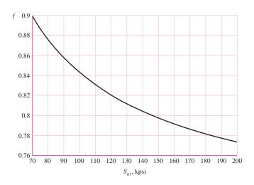
The process given for finding f can be repeated for various ultimate strengths. Figure 6–18 is a plot of f for  $70 \le S_{ut} \le 200$  kpsi. To be conservative, for  $S_{ut} < 70$  kpsi, let f = 0.9.
