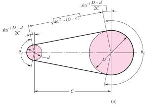
$$\begin{aligned} \theta_d &= \pi - 2 \sin^{-1} \frac{D - d}{2C} \\ \theta_D &= \pi + 2 \sin^{-1} \frac{D - d}{2C} \\ L &= \sqrt{4C^2 - (D - d)^2} + \frac{1}{2} (D\theta_D + d\theta_d) \end{aligned}$$
