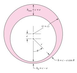
that flows out both ends; the elemental side flow at any position  $\theta$  (Fig. 12–30) is
