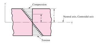
The bending stress varies linearly with the distance from the neutral axis, *y*, and is given by
