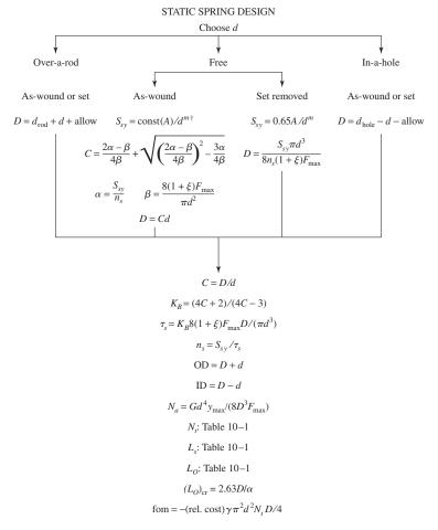
Print or display: d, D, C, OD, ID,  $N_a$ ,  $N_t$ ,  $L_s$ ,  $L_O$ ,  $(L_O)_{\rm cr}$ ,  $n_s$ , fom Build a table, conduct design assessment by inspection Eliminate infeasible designs by showing active constraints Choose among satisfactory designs using the figure of merit
