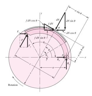
where b is the face width (perpendicular to the paper) of the friction material. Substituting the value of the pressure from Eq. (16-1), the normal force is
