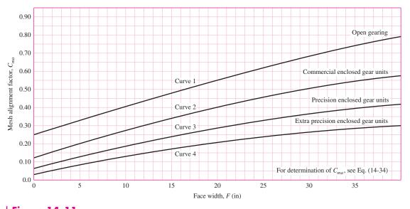
**Figure 14–11**Mesh alignment factor  $C_{ma}$ . Curve-fit equations in Table 14–9. (ANSI/AGMA 2001-D04.)
