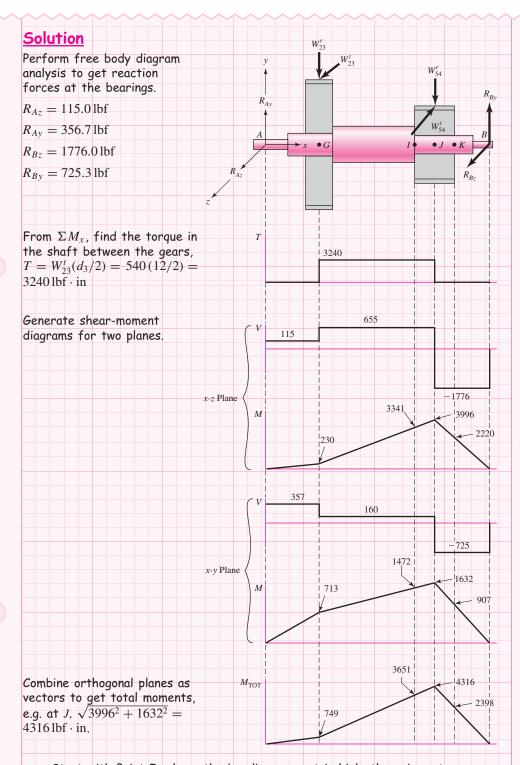
Start with Point I, where the bending moment is high, there is a stress concentration at the shoulder, and the torque is present.
