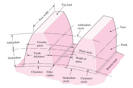
The module m is the ratio of the pitch diameter to the number of teeth. The customary unit of length used is the millimeter. The module is the index of tooth size in SI.
