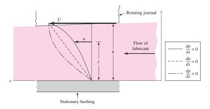
Notice, in the second condition, that h is a function of x. Substituting these conditions in Eq. (e) and solving for the constants gives
