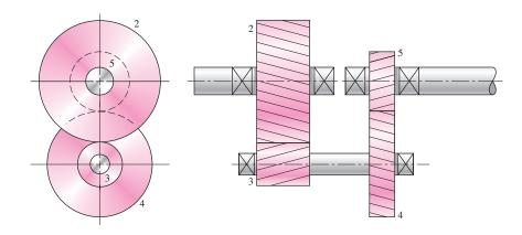
The diametral pitch relates the diameters and the numbers of teeth, P = N/d. Replacing all the diameters gives
