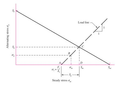
maximum force P. This would be the situation in a pressure cylinder, for example, where a pressure either exists or does not exist. For such cases,  $F_{\text{max}} = F_b$  and  $F_{\text{min}} = F_i$  and the alternating component of the force is  $F_a = (F_{\text{max}} - F_{\text{min}})/2 = (F_b - F_i)/2$ . Dividing this by  $A_t$  yields the alternating component of the bolt stress. Employing the notation from Sec. 8–7 with Eq. (8–24), we obtain
