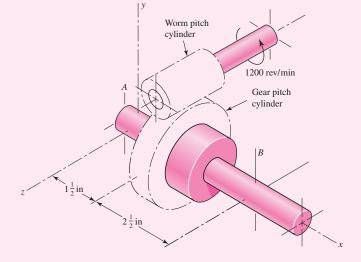
Solution (a) The axial pitch is the same as the transverse circular pitch of the gear, which is
