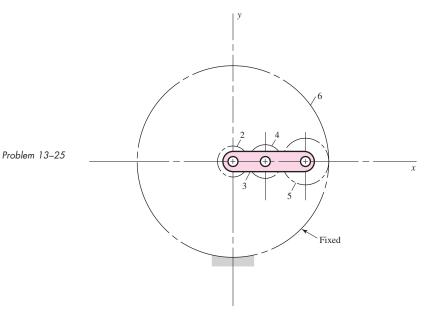
The gears shown in the figure have a diametral pitch of 2 teeth per inch and a 20° pressure angle. The pinion rotates at 1800 rev/min clockwise and transmits 200 hp through the idler pair to gear 5 on shaft *c*. What forces do gears 3 and 4 transmit to the idler shaft?
