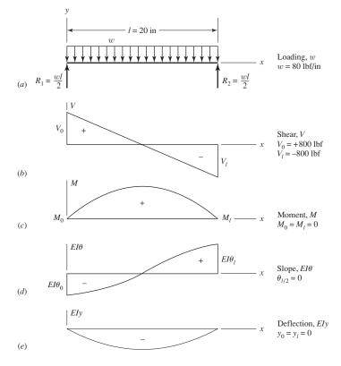
The nomenclature and conventions are illustrated by the beam of Fig. 4–2. Here, a beam of length l=20 in is loaded by the uniform load w=80 lbf per inch of beam length. The x axis is positive to the right, and the y axis positive upward. All quantities—loading, shear, moment, slope, and deflection—have the same sense as y; they are positive if upward, negative if downward.
