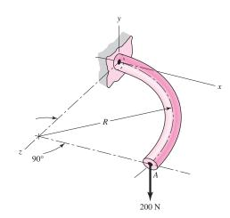
**4–68** For the wire form shown, determine (a) the reactions at points A and B, (b) how the bending moment varies along the wire, and (c) the deflection of the load F. Assume that the entire energy is described by Eq. (4–28).
