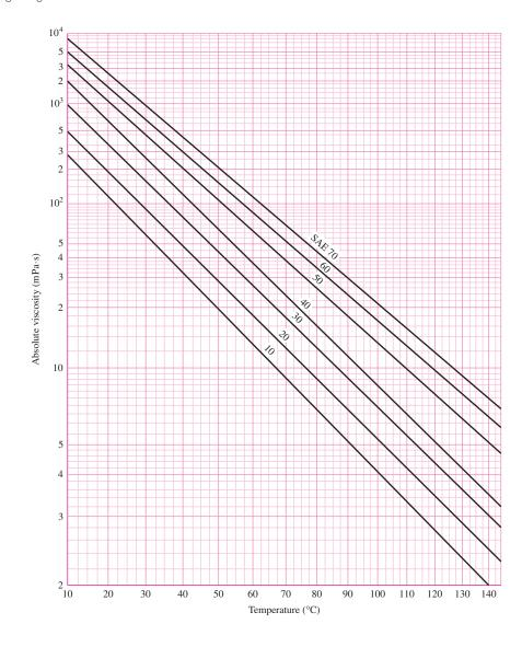
This corresponds to point *A* on Fig. 12–12, which is above the SAE 30 line and indicates that the viscosity used in the analysis was too high.
