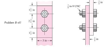
**8-42** The bolted connection shown in the figure is subjected to a tensile shear load of 20 kip. The bolts are SAE grade 5 and the material is cold-drawn AISI 1015 steel. Find the factor of safety of the connection for all possible modes of failure.
