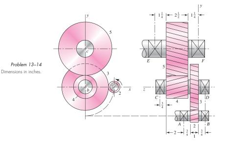
normal pressure angle of  $20^{\circ}$ . The second pair of gears in the train, gears 4 and 5, have a normal diametral pitch of 6 teeth/in, a  $25^{\circ}$  helix angle, and a normal pressure angle of  $20^{\circ}$ . The tooth numbers are:  $N_2 = 14$ ,  $N_3 = 54$ ,  $N_4 = 16$ ,  $N_5 = 36$ . Find:
