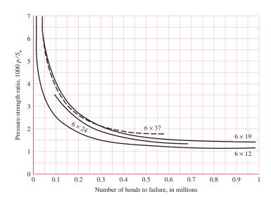
in fatigue or in wear. However, the graph does show that the rope will have a long life if the ratio  $p/S_u$  is less than 0.001. Substitution of this ratio in Eq. (17–42) gives
