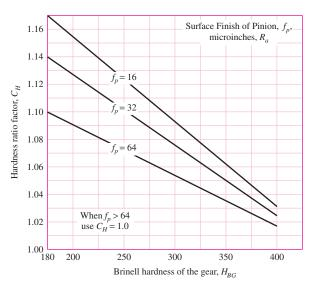
where  $B' = 0.00075 \exp[-0.0112 f_P]$  and  $f_P$  is the surface finish of the pinion expressed as root-mean-square roughness  $R_a$  in  $\mu$  in.
