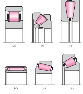
The spherical-roller thrust bearing (Fig. 11-3b) is useful where heavy loads and misalignment occur. The spherical elements have the advantage of increasing their contact area as the load is increased.
