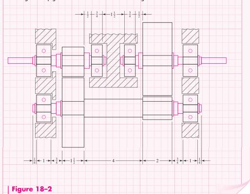
Wider face widths on gears require more shaft length. Originally, gears with hubs were considered for this design to allow the use of set screws instead of high-stress-concentration retaining rings. However, the extra hub lengths added several inches to the shaft lengths and the gearbox housing.
