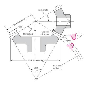
where the subscripts P and G refer to the pinion and gear, respectively, and where  $\gamma$  and  $\Gamma$  are, respectively, the pitch angles of the pinion and gear.
