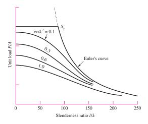
yield strength of 40 kpsi. Note how the P/A contours asymptotically approach the Euler curve as l/k increases.
