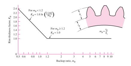
Figure 14–16 also gives the value of  $K_B$  graphically. The rim-thickness factor  $K_B$  is applied in addition to the 0.70 reverse-loading factor when applicable.
