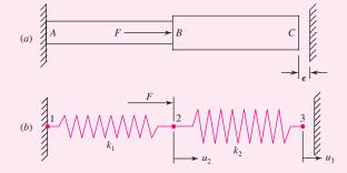
reactions, the internal forces in the members, and the deflection of point B. Let E=10 Mpsi and assume that end C hits the wall. Check the validity of the assumption.
