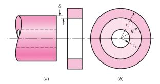
With p, Eq. (3–49) can be used to determine the radial and tangential stresses in each member. For the inner member,  $p_o = p$  and  $p_i = 0$ , For the outer member,  $p_o = 0$  and  $p_i = p$ . For example, the magnitudes of the tangential stresses at the transition radius R are maximum for both members. For the inner member
