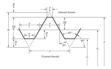
larger minor diameter of both the internal and external threads. This profile is especially useful where high fatigue strength is required.
