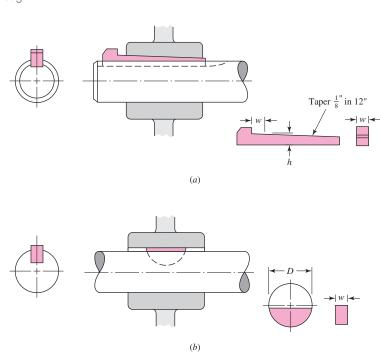
The gib-head key, in Fig. 7–17*a*, is tapered so that, when firmly driven, it acts to prevent relative axial motion. This also gives the advantage that the hub position can be adjusted for the best axial location. The head makes removal possible without access to the other end, but the projection may be hazardous.
