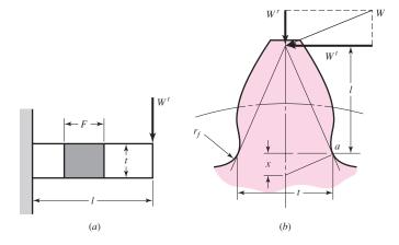
Referring now to Fig. 14–1b, we assume that the maximum stress in a gear tooth occurs at point a. By similar triangles, you can write
