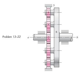
**13–23** The tooth numbers for the gear train illustrated are  $N_2 = 24$ ,  $N_3 = 18$ ,  $N_4 = 30$ ,  $N_6 = 36$ , and  $N_7 = 54$ . Gear 7 is fixed. If shaft *b* is turned through 5 revolutions, how many turns will shaft *a* make?
