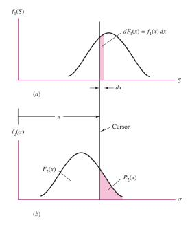
designate the strength distribution and the subscript 2 to designate the stress distribution. Figure 5–32 shows these two distributions aligned so that a single cursor x can be used to identify points on both distributions. We can now write
