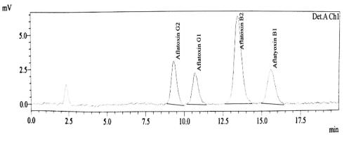
Figure 1. Chromatogram for intensity against retention time for the standard used for aflatoxins analysis
