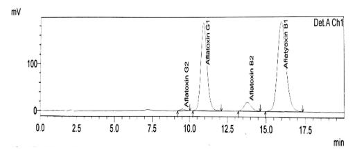
Figure 2. Chromatogram for intensity against retention time for one of the samples analysed for aflatoxins
