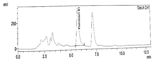
Figure 6. Chromatogram for intensity against retention time for one of the samples analysed for fumonisins
