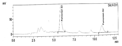
Figure 5. Chromatogram for intensity against retention time for the standard used for fumonisins analysis
