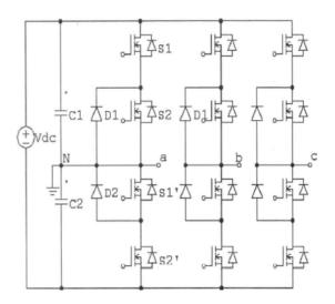
Fig. 1 Diode Clamped Three Level Inverter
