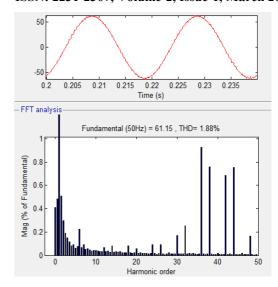
Fig 8. Harmonic of spectrum Line current of 3-level inverter for R= 15, L=24.2 mH  $\,$
