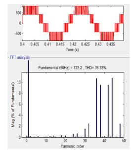
Fig 7. Harmonic spectrum Line Voltage of 3-level inverter for R= 15, L=24.2 mH
