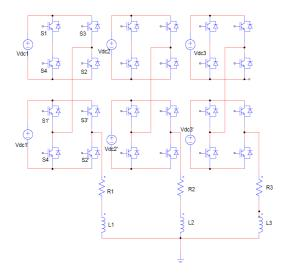
Fig. 3 Cascaded Inverters with Separate DC Source
