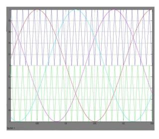
Fig 4. Control Pulse Generation in Three Level SPWM
