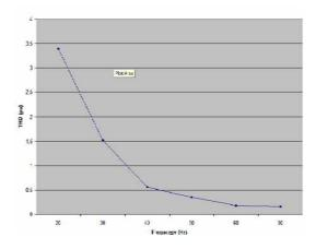
Fig. 9 Effect of Inverter o/p Frequency on Load Current THD for Fixed RL
