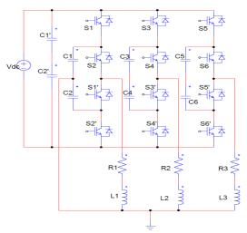
Fig. 2 Flying Capacitor Three Level Inverter
