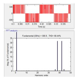
Fig 5. Harmonic Spectrum of Line Voltage of 2-level inverter for R= 15, I = 24.2 mH
