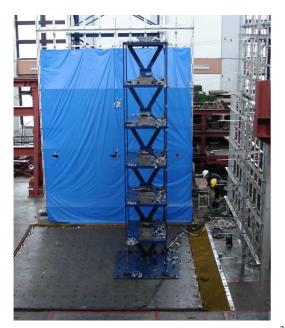
Figure 3 Six-story test structure mounted to the 25  $m^2$  shaking table at the National Center for Research on Earthquake Engineering (NCREE), Taipei, Taiwan
