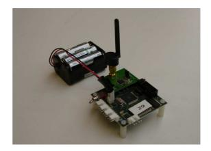
Figure 2 Narada wireless sensing and actuation node
