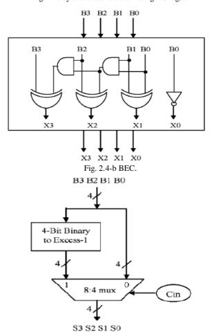
Fig. 3. 4-b BEC with 8:4 mux.
