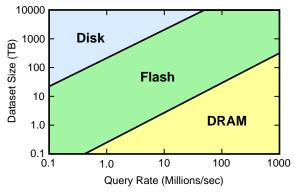
**Figure 2.** This figure (reproduced from Andersen et al. [1]) indicates which storage technology has the lowest total cost of ownership over 3 years, including server cost and energy usage, given the required dataset size and query rate for an application (assumes random access workloads).
