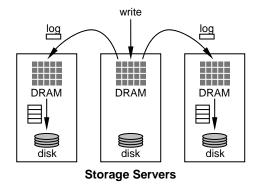
**Figure 3.** In the buffered logging approach to durability, a single copy of each object is stored in DRAM. When an object is modified, the changes are logged to 2 or more other servers. Initially the log entries are stored in the DRAM of the backup servers; they are transferred to disk asynchronously in batches in order to utilize the full disk bandwidth.
