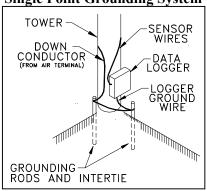
Their dimensions will determine the contact surface area with the soil, a key element for proper system grounding. A combination of the three can be used to enhance the contact area if they are all electrically connected.
