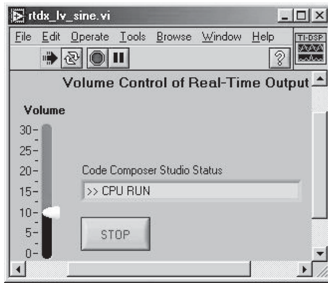
FIGURE 9.33. LabVIEW Instrument window for controlling the DSK output amplitude of a sine wave through RTDX for the project rtdx_lv_sine .
