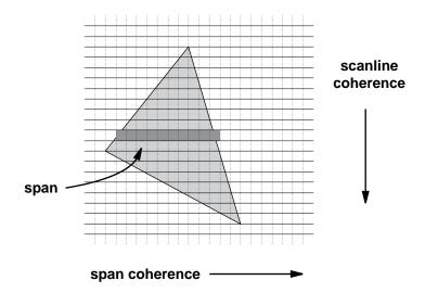
**Figure 5. Spatial coherence in image space.** Pixel values tend to be similar from one scanline to the next, and from pixel to pixel within spans. Sequential rendering algorithms exploit this property to reduce computation costs during scan conversion.
