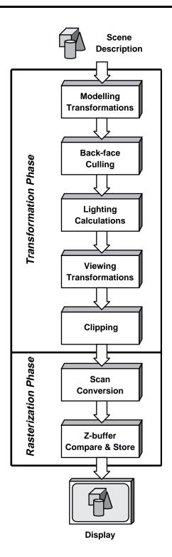
Figure 2. A typical polygon rendering pipeline. The number of function units and their order varies depending on details of the implementation.
