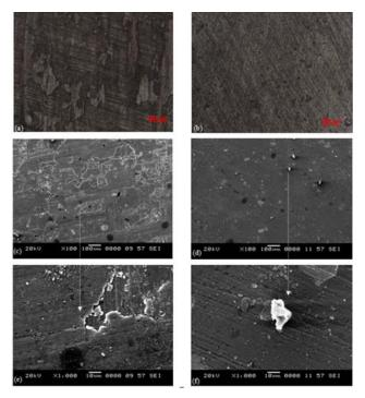
**Figure 8.** Wear test image of AlCrN deposited on (a) Optical of EN353/4µm; (b) Optical of EN31/4µm; (c) SEM of EN353/4µm; (d) SEM of EN31/4µm; (e) SEM of close-up view of EN353/4µm and (f) SEM of close-up view of EN31/4µm
