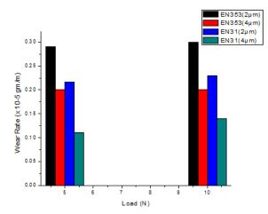
Figure 7. Measurement of wear rate for different coating thickness and carbon contents of the substrate
