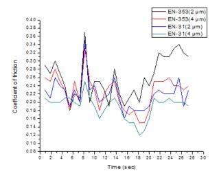
Figure 6. Variation of coefficient of friction vs stroke length for different coating thicknesses and carbon Contents of the substrate.
