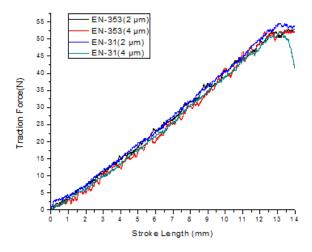
Figure 4. Variation of traction force vs stroke length for different coating thicknesses and carbon contents of the substrate.
