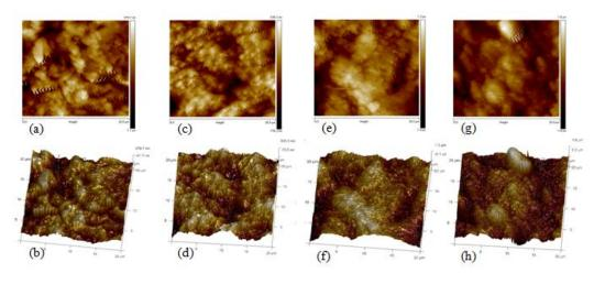
Figure 2. 2D and 3D AFM images of AlCrN coating deposited on EN353 (2µm (a, b) & 4µm (e, f)) and EN31 steel (2µm(c, d) & 4µm(g, h)).
