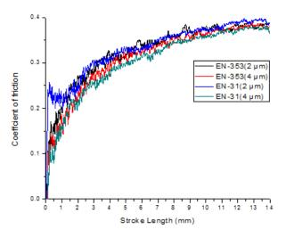
Figure 3. Variation of coefficient of friction vs stroke length for different coating thicknesses and carbon contents of the substrate
