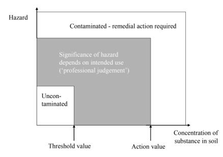
Figure 1: Interpretation of ICRCL trigger concentrations (redrawn from ICRCL, 1987).
