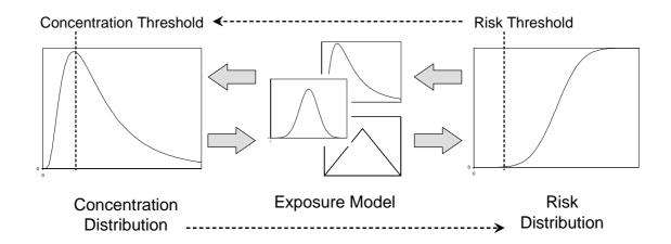
Figure 2: Schematic QRA modelling procedures. In practice, probabilistic exposure models can be used to calculate distributions of risk associated with distributions of environmental (eg. soil) contaminants, or they can back-calculate concentration thresholds from pre-determined risk thresholds.
