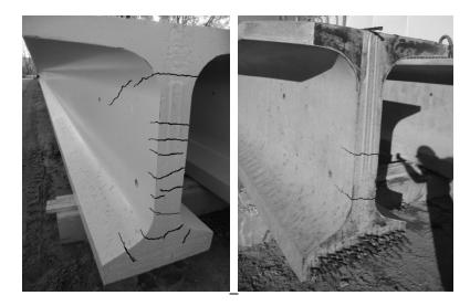
Figure 11 - Cracks on a girder with 0% (left) and 43% (right) debonded strands.
