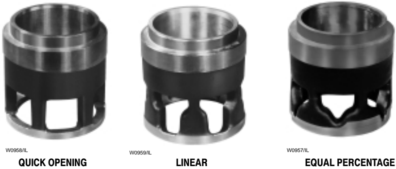
Figure 3-27. Characterized Cages for Globe-Style Valve Bodies
