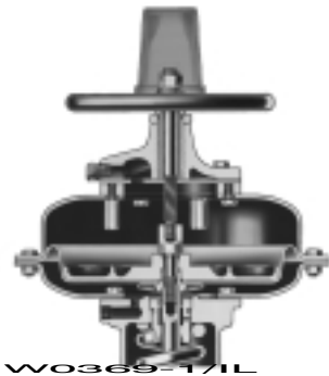
Figure 4-6. Top-Mounted Hand-wheel for Reverse-Acting Diaphragm Actuator
