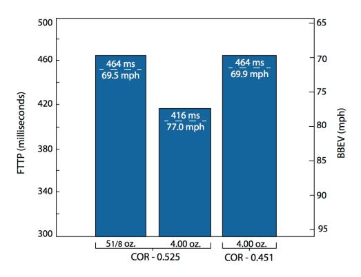
**Figure 2.2** Relationship between ball mass, COR, FTTP, and BBEV. A fourounce ball will reach the pitcher 48 ms faster than a standard ball while a four-ounce ball with a reduced COR will reach the pitcher in same amount of time.
