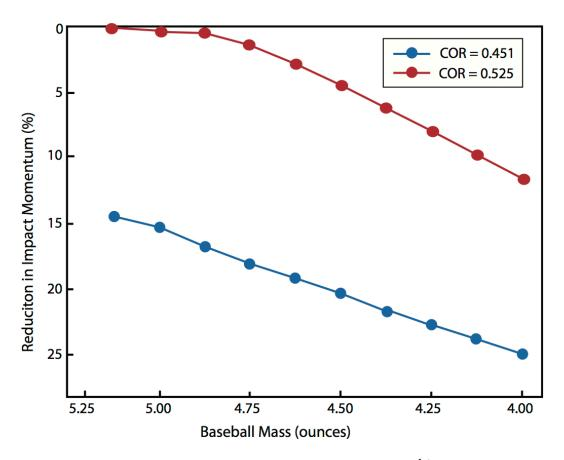
**Figure 2.3** The reduction in impact momentum compared to a 5 1/8 ounce ball with a COR of 0.525. A four-ounce ball sees a 15% reduction in impact momentum while a four-ounce ball with reduced COR sees a 25% reduction in impact momentum.
