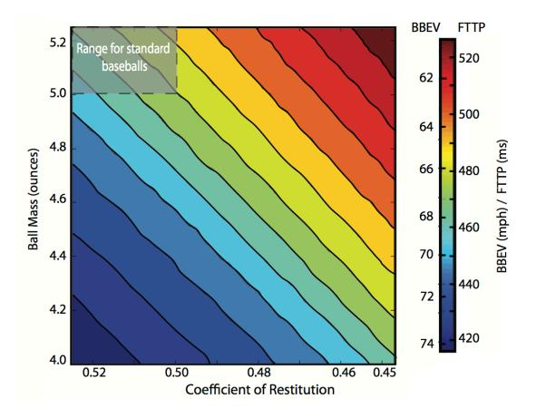
**Figure 2.5** A contour plot of BBEV and FTTP for balls of varying mass and COR. As ball mass and COR are reduced, FTTP and BBEV can be consistent with a standard ball.
