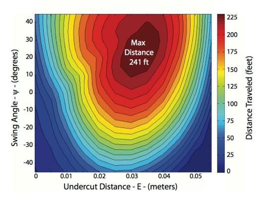
**Figure 2.4** A contour plot of batted ball range for a standard ball under varying unique swing conditions. The maximum range for a standard ball is 241 feet.
