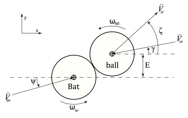
**Figure 2.1** Two-dimensional impact schematic adapted from Sawicki et al. Impact occurs with horizontal, vertical and rotational bat and ball velocities. Post-impact variables that control trajectory include  $\hat{V}_{bf}$ ,  $\omega_{bf}$ , and  $\zeta$ .
