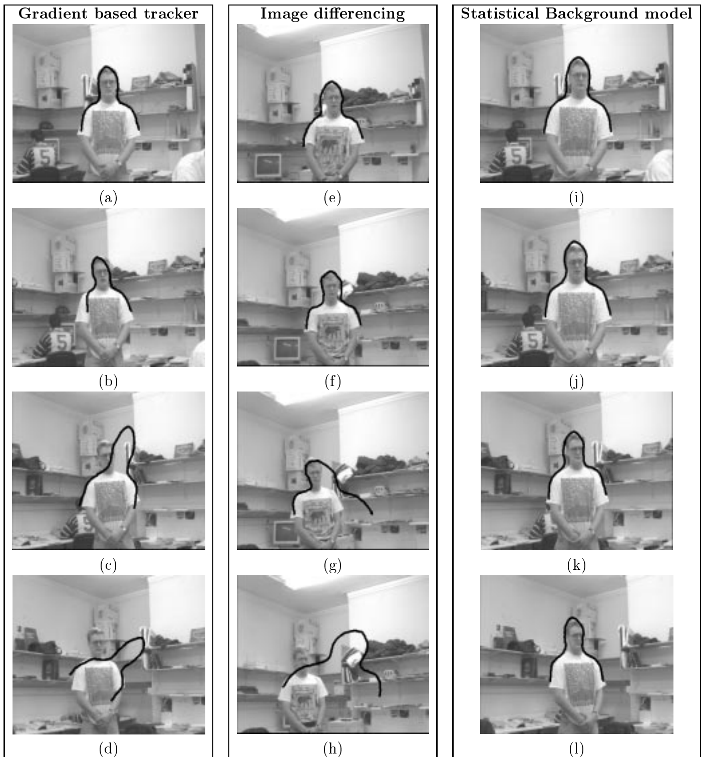
Figure 2: In the left-hand sequence ((a) - (d)), a gradient-based feature detector is used to track a target as it moves across a room. The camera is mounted on a pan-tilt head. Because the foreground is fixated it appears stationary, but note how the background moves relative to the target. As the target passes some strong clutter the contour is distracted ((c) and (d)) and loses track of the target. The middle column((e)-(h)) shows a similar tracking sequence, but using image differencing. The contour is still distracted by the edges of objects in the background and loses track of the target (h). Finally, in the right hand column, the background has been modelled statistically on the virtual image plane. Edges in the background are ignored (k) enabling tracking to continue past the clutter (l).
