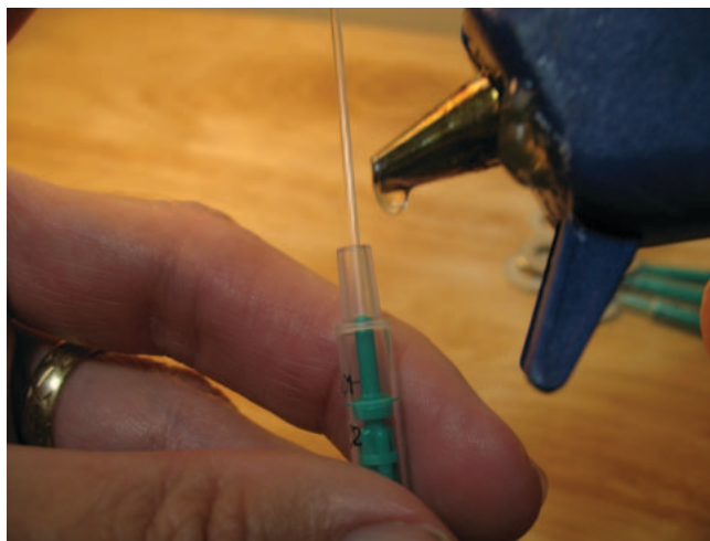
Figure 3. Hot Glue Added to Capillary Tube Base
