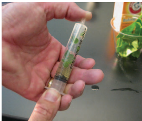
Figure 6a. Creating a Vacuum in the Plunger
