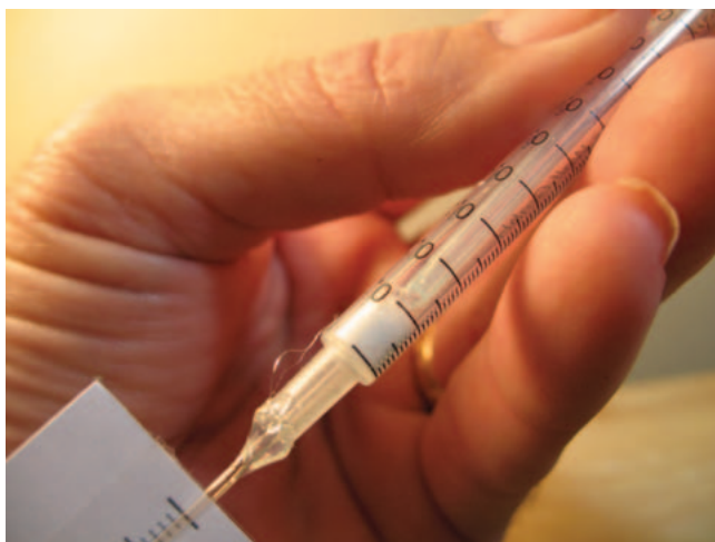
Figure 4. Cotton Inserted into Microrespirometer Barrel
