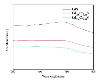
Figure 1. Absorption spectra for  $Cd_{1-x}Co_xS$  (x = 0, 0.02 and 0.04)
