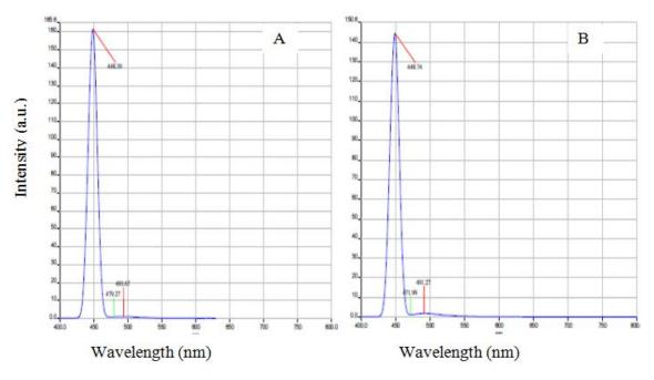
Figure 4. Photoluminescence (PL) spectra of Ni-doped CdS with doping concentration 2% (A) and 4% (B)
