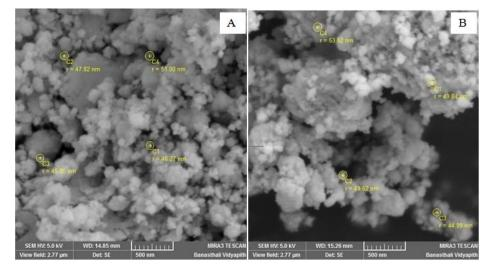
Figure 6. SEM imagea of Ni-doped CdS with doping concentration 2% (A) and 4% (B)
