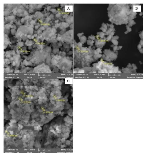
Figure 5. SEM images of undoped CdS (A) and Co-doped CdS with doping concentration 2% (B) and 4% (C)
