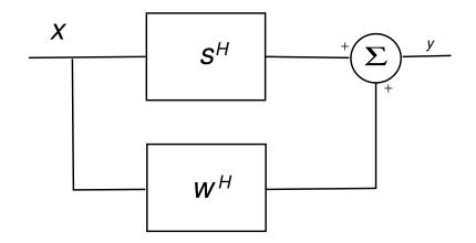
Figure 7: Block diagram of the minimum output energy formulation
