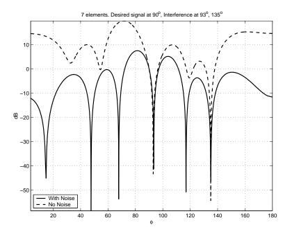
Figure 4: Adapted pattern with and without noise.
