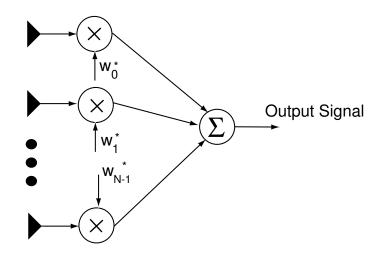
Figure 1: A general beamforming system.
