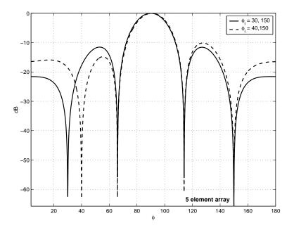
Figure 2: Illustration of nulling using the optimal beamformer.
