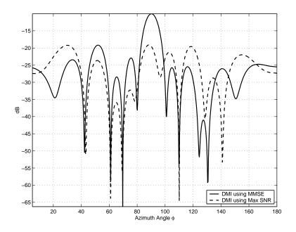
Figure 6: Adapted beampattern using the MMSE and Max SNR techniques.
