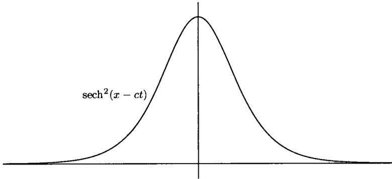
Figure 4.1: Plot of a Solitary Wave Solution
