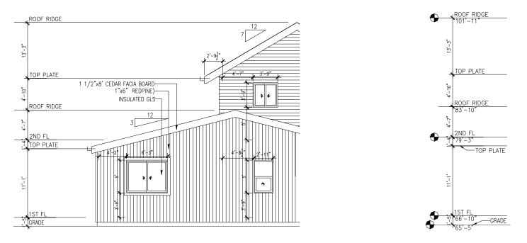
Figure 41. Dimensioning exterior elevations 1
