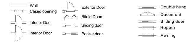
Figure 7, Walls & doors symbols in plan view
