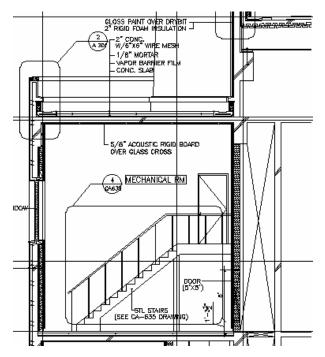
Figure 20. Detail symbol used on the section view
