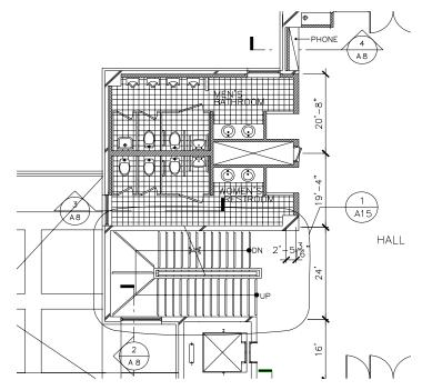
Figure 19. Detail symbol used on the plan view
