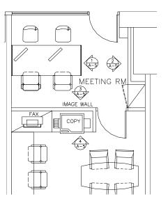
Figure 16. Elevation symbol used on the plan view
