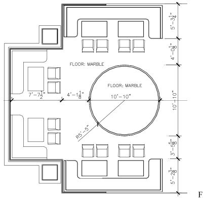
Figure31 Dimensioning a curve
