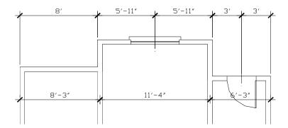
Figure 32. Dimensioning frame buildings
