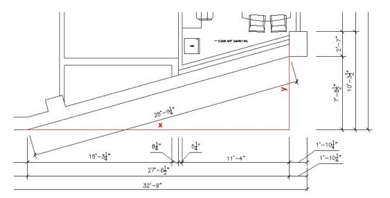
Figure 30. An example of dimensioning an angled wall along an *x* and a *y* axis.
