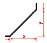
Figure 29. Dimensioning an angled wall
