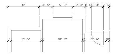
Figure 33. Dimensioning concrete/ masonry buildings
