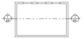
Figure 3. Section symbols and lines placed on a drawing
