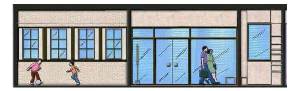
Figure39 Adding people on interior elevation drawings gives a relative sense of object heights
