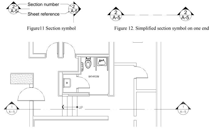
Figure 13. Section symbols used on the plan view
