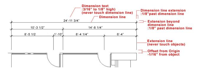
Figure 28. Dimension techniques for floor plans
