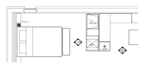
Figure 17. Multiple elevation symbol used on the plan view
