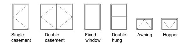
Figure 10. Examples of window symbols in elevation view
