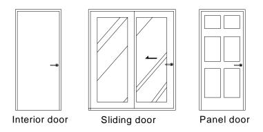
Figure 9. Examples of door symbols in plan view
