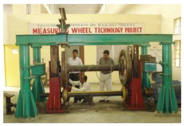
**Measuring Wheel Experimental Setup**
