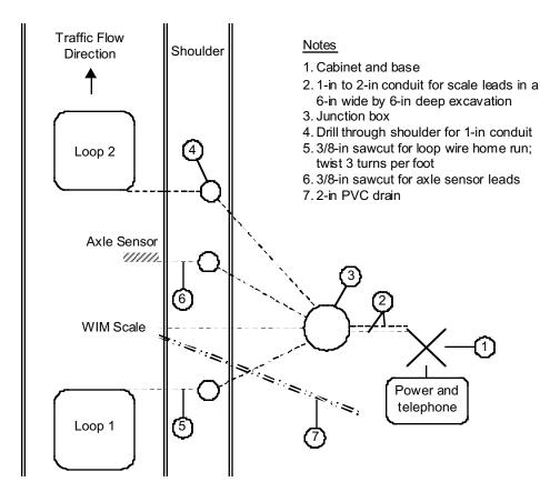
Figure 12. Bending plate or load cell WIM system (typical).
