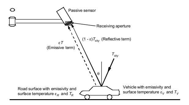
Figure 27. Emission and reflection of energy by vehicle and road surface.
