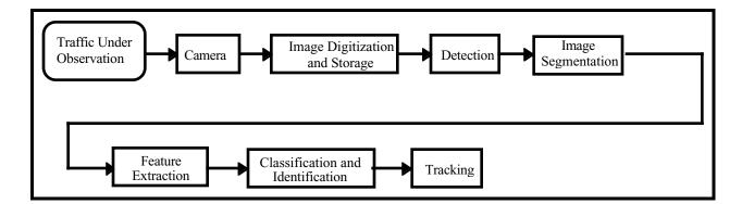
Figure 17. Conceptual image processing for vehicle detection, classification, and tracking.
