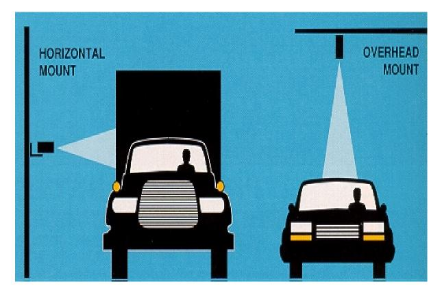
Figure 30. Mounting of ultrasonic range-measuring sensors. (Courtesy of Microwave Sensors, Ann Arbor, MI).
