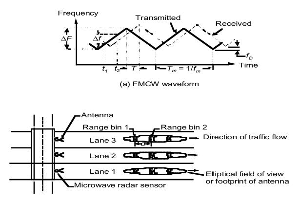
(b) Range binned footprints of radar sensors in traffic lanes
