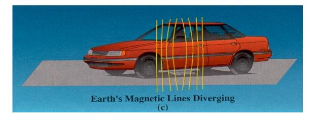
Figure 8. Distortion of Earth's magnetic field created as a vehicle enters and passes through the detection zone of a magnetic sensor. (Drawing courtesy of Nu-Metrics, Vanderbilt, PA).
