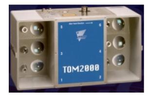
(b) Traffic observation module (TOM) laser radar sensor. (Photograph courtesy of MBB SensTech, Munich, Germany).
