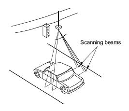
Figure 24. Laser radar beam geometry. (Drawing courtesy of Schwartz Electro-Optics, Orlando, FL).
