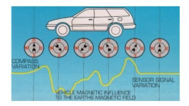
(b) Perturbation of Earth s magnetic field by a ferrous metal vehicle. (Drawing courtesy of Nu-Metrics, Vanderbilt, PA).
