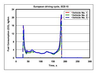
Figure 12. Time history of fuel consumption due to carbon monoxide (CO)
