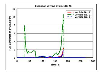
Figure 11. Time history of fuel consumption due to nitrogen oxide (NO<sub>x</sub>)
