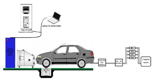
Figure 2. Overview of the laboratory chassis dynamometer test
