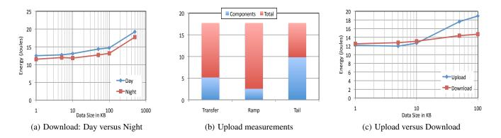
Figure 4: 3G Measurements: (a) Comparison of average energy consumption of day versus night time downloads of 50K data.(b) Average transfer, tail and ramp energy consumed for uploading 50K data (c) Comparing the average energy consumed for downloading 50K data versus uploading 50K data.
