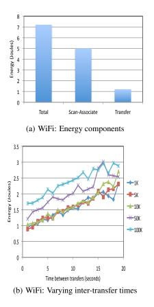
Figure 7: WiFi Measurements: (a) Average scan/associate and transfer energy consumed to download 50K data. The lower portion of the stacked columns show the proportion of energy spent for each activity compared to the total energy spent. (b) Averagenergy consumed for downloading data of different sizes against the inter-transfer time.
