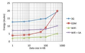
Figure 8: : WiFi versus 3G versus GSM measurements: Average energy consumed for downloading data of different sizes against the inter-transfer time
