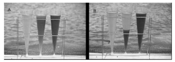
Figure 12. (A) Clarifier effluent from culture tank water, (B) Sludge from clarifier after 10 minutes settling.
