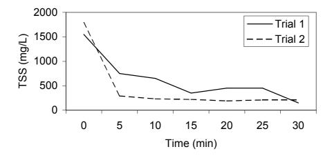
Figure 11. TSS settling curve - Trials 1 and 2.
