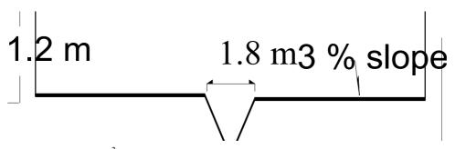
Figure 1. A 200-m<sup>3</sup> rearing tank with center cone and external drain line.
