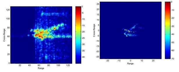
Fig. 7 ISAR imaging from normal motion Fig. 8 ISAR image from the EM model compensation
