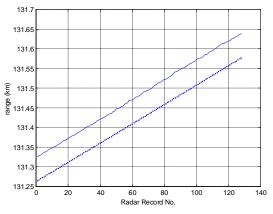
Fig. 2 GPS range (solid) vs. radar track range (dotted)
