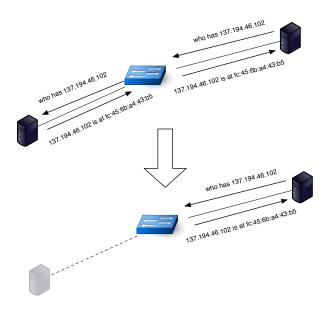
Fig. 4. External proxying: a switch acts as a proxy for ARP traffic, allowing the target machine to sleep at least until data traffic is sent.
