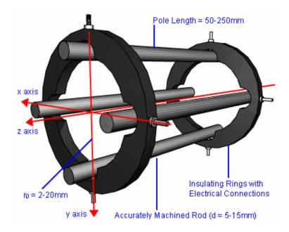
Where the ion is caused to oscillate with a trajectory whose amplitude exceeds  $r_0$  it will collide with a rod, and become discharged and subsequently pumped to waste. This is known as an unstable or collisional trajectory.
