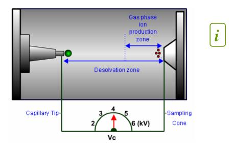
Sprayed eluent droplet –desolvated using heated drying gas within the interface.
