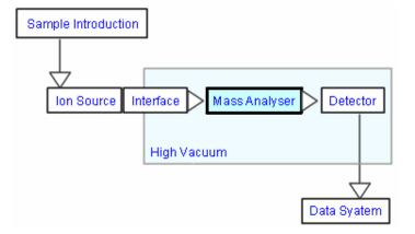
There are several very popular types of mass analyser associated with routine liquid chromatography mass-spectrometric analysis and all differ in the fundamental way in which they separate species on a mass-to-charge basis:
