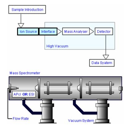
Where the "Flow rate" label denotes the effluent (analyte plus eluent and additives) coming from the HPLC system.
