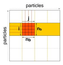
Figure 2: Schema of the splitting of the force calculation into blocks. Each of the  $n_b$  threads is dedicated to calculating all interactions of particle i. All particles j are loaded in blocks of again  $n_b$  particles, which are then shared among all threads.
