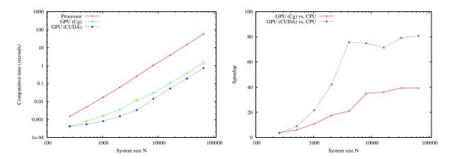
Figure 3: Left: Time (in seconds) required to integrate a single MD time step as a function of system size N. Right: Speedup factor for both GPU implementations, Cg and CUDA. The speedup saturates once both the processor and GPU versions have reached the quadratic scaling regime.
