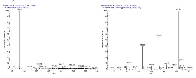
Figure 5. a) ESI spectrum of nicotine from tobacco extraction; b) ESI-ms/ms spectra of peak at 163.04 and fragmentation patterns of nicotine
