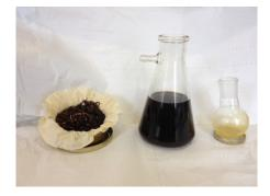
Figure 1. From the left: tobacco leaves, basic solution for extraction, concentrate solution containing nicotine
