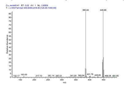
Figure 9. ESI-MS/MS spectra of the peak at m/z= 448.69 and fragmentation patterns (loss of a nitrate)
