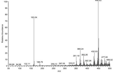
Figure 8. ESI spectrum of Cu-nicotine solution from the green solution obtained in the qualitative experiment
