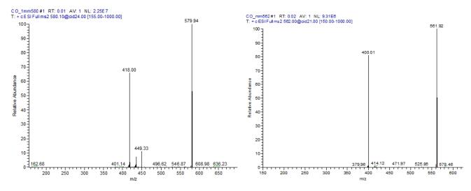
Figure 7. ESI-MS/MS spectra of Co-NIC complexes. On the left: ESI-MS/MS spectra of the peak at m/z=580 and fragmentation patterns (loss of a nicotine ligand); on the right: ESI-MS/MS spectra of the peak at m/z=561 and fragmentation patterns (loss of a nicotine ligand)
