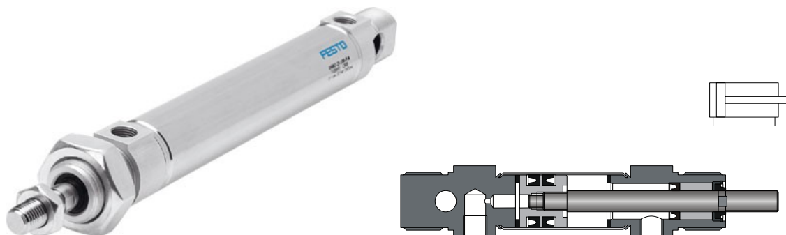
Figure 5.5: Picture, sectional view and circuit diagram of a double-acting cylinder
