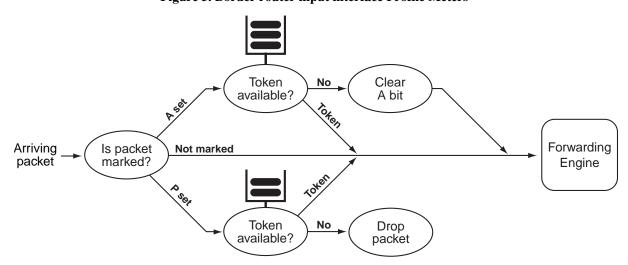
Figure 5. Border router input interface Profile Meters
