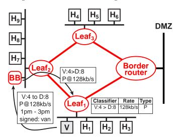
Figure 6. Bandwidth Broker setting Profiles in leaf routers
