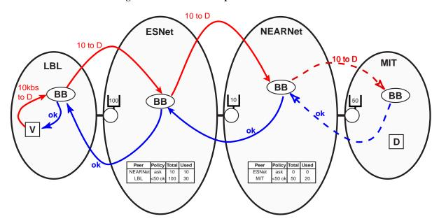
Figure 7. End-to-end example with static allocation.
