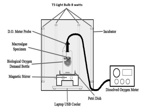
Figure 1. Schematic diagram of the incubating chamber
