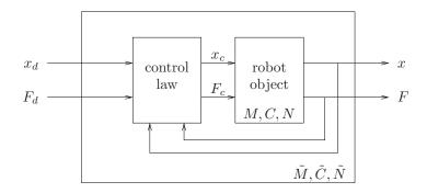
Figure 6.12: Data flow in a typical controlled robot.
