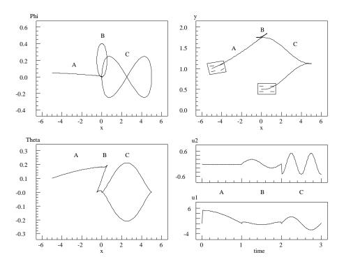
Figure 8.1: Sample trajectories for the motion of a car. The trajectory shown is a sample path which moves the car from  $(x, y, \theta, \phi) = (-5, 1, 0.05, 1)$  to (0, 0.5, 0, 0). The first three figures show the states versus x, the bottom right graphs show the inputs as functions of time.
