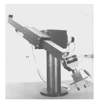
Figure 1.1: The Stanford manipulator. (Courtesy of the Coordinated Science Laboratory, University of Illinois at Urbana-Champaign)
