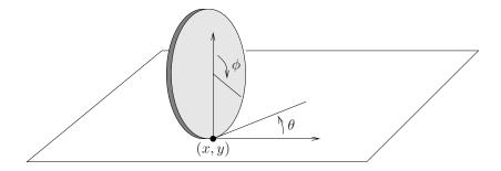
Figure 6.2: Disk rolling on a plane.
