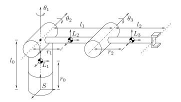
Figure 4.5: Three-link, open-chain manipulator.
