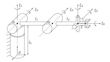
Figure A.2: An elbow manipulator
