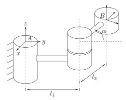
Figure 2.6: Rigid body displacement generated by rotation about a fixed axis.
