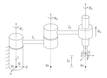
Figure 3.3: SCARA manipulator in its reference configuration.
