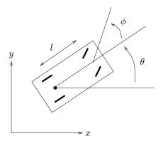
Figure 7.8: Kinematic model of an automobile.
