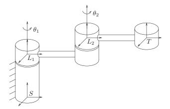
Figure 3.2: A two degree of freedom manipulator.
