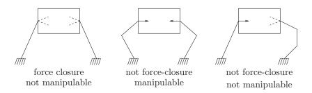
Figure 5.16: Some grasps illustrating manipulability and force-closure properties.
