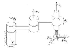
Figure 3.15: End-effector wrenches which generate no joint torques.
