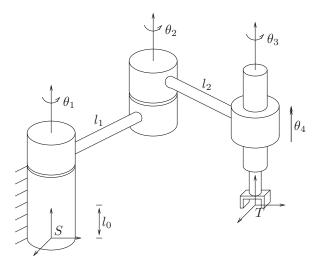
Figure 3.13: SCARA manipulator in non-reference configuration.
