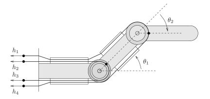
Figure 6.9: Planar tendon-driven finger.
