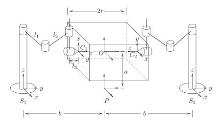
Figure 6.6: Two-fingered grasp using SCARA robots.
