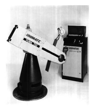
Figure 1.3: The Unimation PUMA (Programmable Universal Manipulator for Assembly). (Courtesy of Stäubli Unimation, Inc.)
