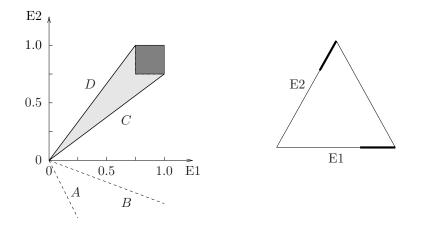
Figure 5.13: Force-closure grasps for an equilateral triangle. The lightly shaded region corresponds to the set of all force-closure grasps and the dark square (and corresponding darkened regions on the triangle) indicates maximally independent regions of contact.
