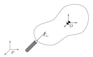
Figure 5.3: Frictionless point contact.
