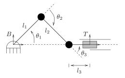
6. Derive the actuator kinematics for the tendon networks shown below. Consider both the rigid and elastic cases.
