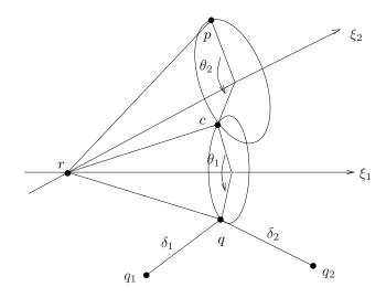
Figure 3.25: Subproblem 4: Rotate p about the axis of  $\xi_1$  followed by a rotation about the axis of  $\xi_2$  such that the final location of p is  $\delta_1$  from  $q_1$  and  $\delta_2$  from  $q_2$ .
