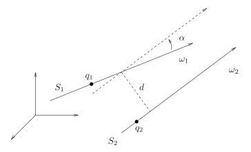
Figure 2.15: Notation for reciprocal screws.
