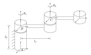
Figure 2.12: Two degree of freedom manipulator.
