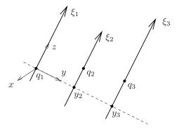
Figure 3.16: Three coplanar, parallel, revolute twists.
