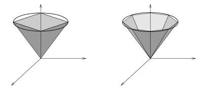
Figure 5.10: Approximations of a spatial friction cone.
