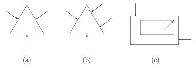
2. Construct the grasp map for the grasps shown below and write the friction cone conditions with respect to the contact basis you choose. Determine if the grasp is force-closure. Assume that all contacts are point contacts with friction.
