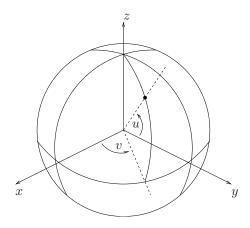
Figure 5.20: Spherical coordinate chart for a sphere.
