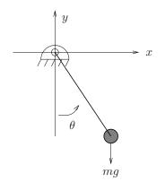
Figure 6.1: Idealized planar pendulum.
