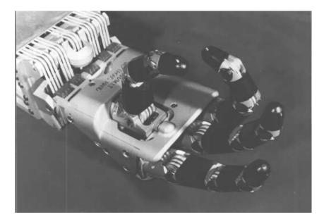
Figure 5.1: The Utah/MIT hand. (Photo courtesy of Sarcos, Inc.)
