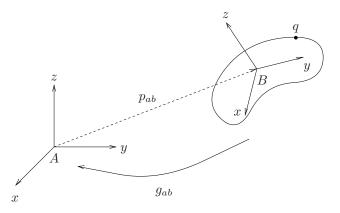
Figure 2.3: Coordinate frames for specifying rigid motions.
