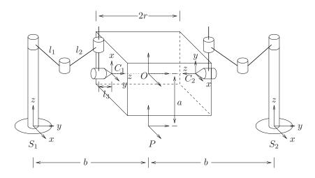
Figure 5.17: Two-fingered grasp using SCARA robots.
