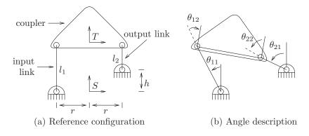
Figure 3.19: Four-bar linkage.
