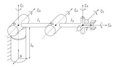
Figure 3.4: Elbow manipulator.
