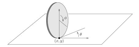
Figure 7.7: Disk rolling on a plane.
