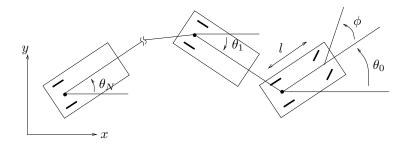
Parameterize the configuration by the states of the automobile plus the angle of each of the trailers with respect to the horizontal. Show that the control equation for the system has the form
