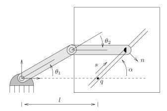
Figure 4.12: Planar manipulator moving in a slot.
