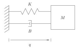
Figure 4.8: Damped harmonic oscillator.
