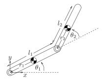
Figure 4.4: Two-link planar manipulator.
