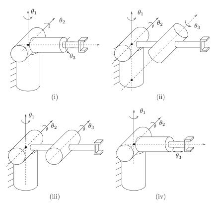
Figure 3.23: Some simple three degree of freedom manipulators.
