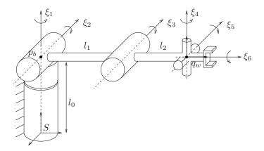
Figure 3.11: Elbow manipulator.
