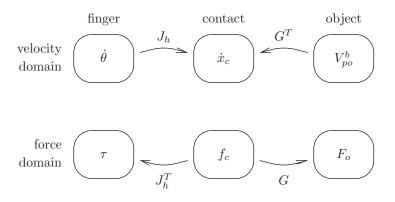
Figure 5.15: Diagram of relationships for a multifingered grasp. The contact force must satisfy  $f_c \in FC$  for these relationships to hold.
