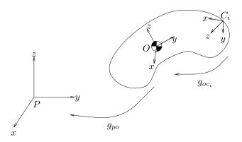
Figure 5.2: Coordinate frames for contact and object forces.
