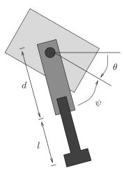
Figure 7.5: A simple hopping robot.
