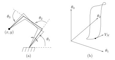
Figure 3.17: Self-motion manifold for a redundant planar manipulator.
