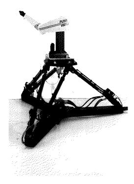
Figure 3.21: A Stewart platform with a PUMA robot attached. (Photo courtesy of Steve Dubowsky, MIT)
