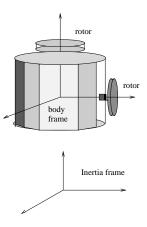
Figure 7.9: A model of a satellite body with two rotors. The satellite can be repositioned by controlling the rotor velocities. (Figure courtesy of Greg Walsh)
