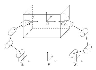
Figure 2.14: Coordinate frames for a simple grasping example.
